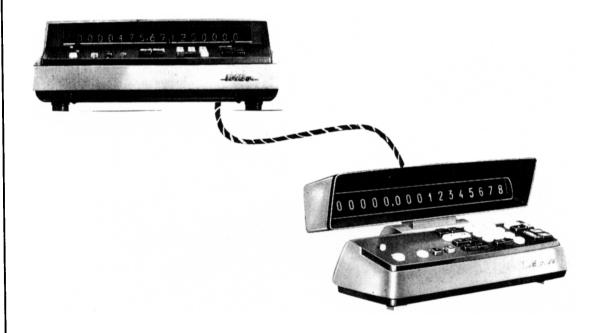
The connection is done by means of a special cable. If more than one keyboard has to be connected, a distribution box is required. IME makes great fanfare with this system, but it is very doubtful if it will prove to be successful in future.
