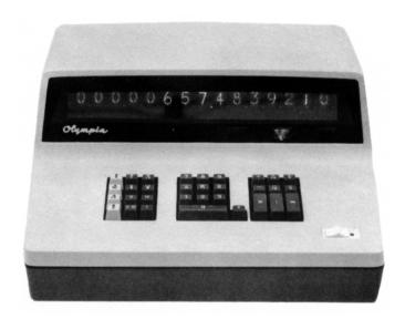
The Olympia 4/15 is operated via a 11 key-keyboard and 21 control keys for arithmetical operations, storing and clearance. Those keys can be split up into 5 different groups:
