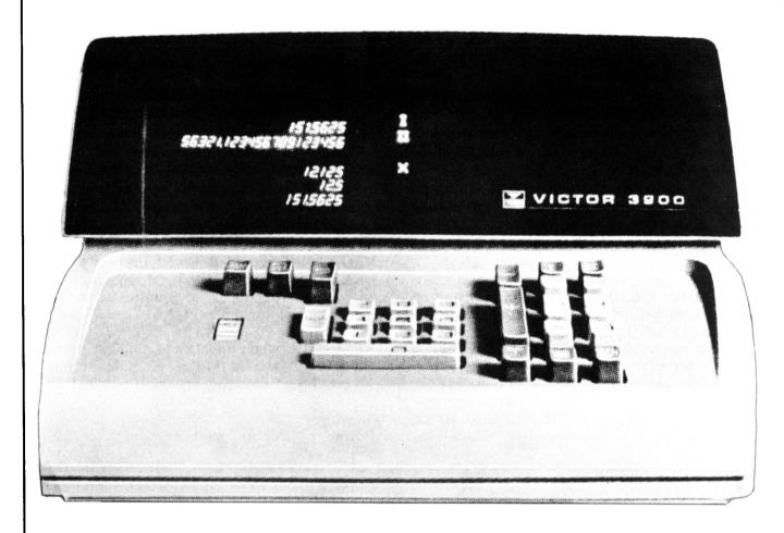
The dimensions of the 3900 are approximately 20" long, 11" wide and 7 - 1/2" high and it weighs 24 pounds. It incorporates an integrated electronic circuit consisting of 30 chips in contrast to the transistorized circuitry found in the 130. It has a cathode ray tube on which five registers may be viewed. However, this calculator does not have the stacking principle which is used in the 130 display.
