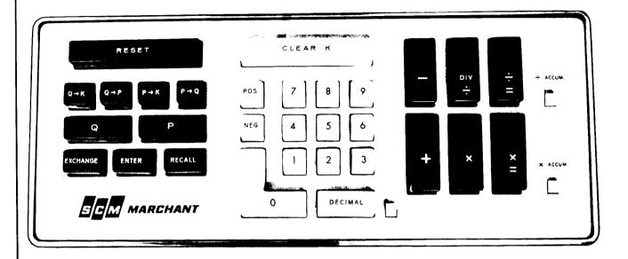
An eleven key keyboard is used for input of all numbers. It includes a decimal point key and an L-shaped zero bar similar to the zero bar on the AFY adding machine. The decimal point key is used whenever a decimal point appaers in a number. It is not used for whole numbers.
