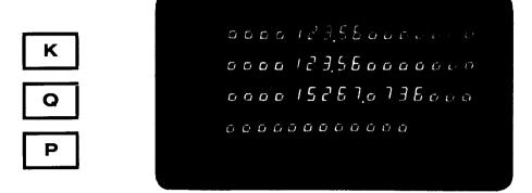
The P register is a combination of the bottom two columns of zeros. The second from the bottom register has 16 zero digits. The first four zero digits are used only as zero digits in decimal answers in the same manner as described for the K register. The bottom register has 12 zero digits with four blank spaces on the right. The total of these two registers provides a combination of 24 usable digits for a product.
