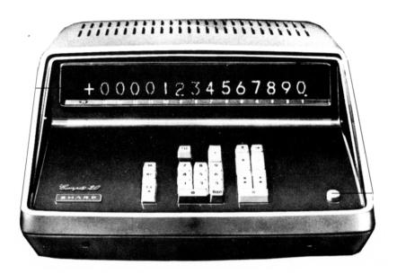
This model which is quite similar to the Canola 130 has a 10 key key-board. It is designed to carry out addition, subtraction, multiplication and division. The machine automatically clears, calculates and prositions the figures, including the decimal point if required.
