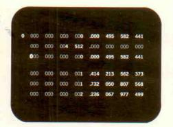
Multiplier-Quotient Register Entry Register Accumulator Register
